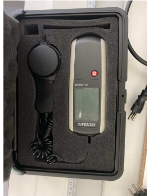
Figure 1.7: A luxmeter measures illuminance, which is the total amount of visible light falling on a surface per unit area. Please do not forget to remove the protective rubber cap before starting the measurement.
